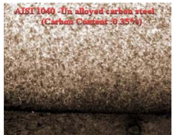
Fig. (7). Case – core interface showing martensite in the case and ferrite/pearlite in the core region.
