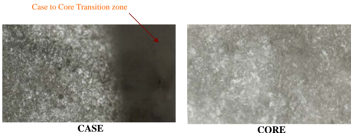
Fig. (5). Microstructure of Case and Core portion of EN 353 pinion material.
