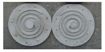
Fig. (5). Soft mold of silicone rubber.
