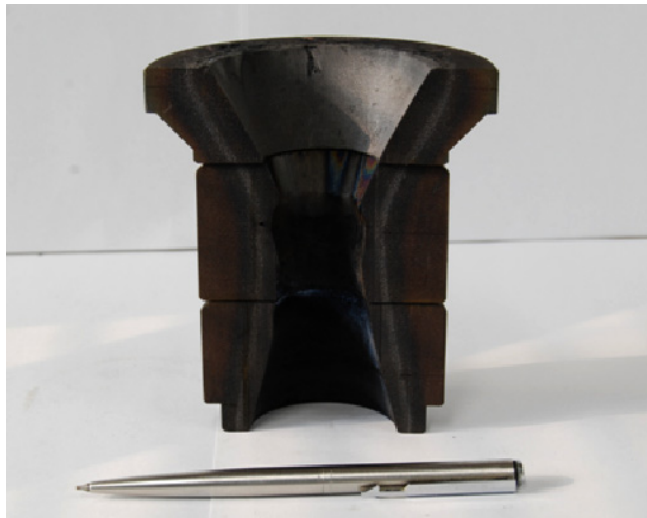
Fig. (12). Nozzle components of rocket motor.
