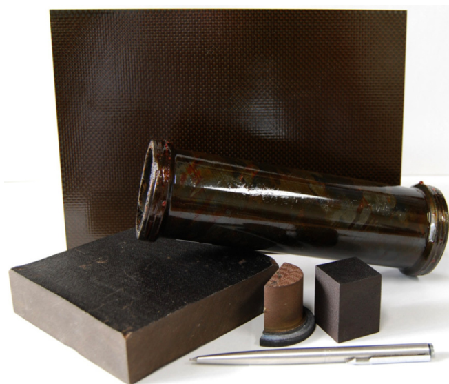
Fig. (7). Fiber-reinforced plastics (FRP) using MSP as a matrix resin.
