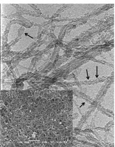
Fig. (2). Scanning and transmission electron microscope images of pristine and acid treated MWCNTs. (a) pristine MWCNT (white arrow: impurities), (b) purified MWCNT, (c) functionalized MWCNT (black arrow: defect generation).
