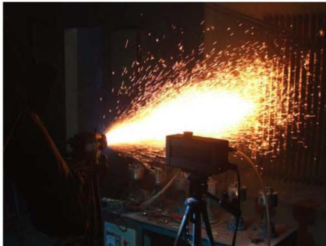
Fig. (14). SprayWatch thermal spraying jet flow inspection device.
