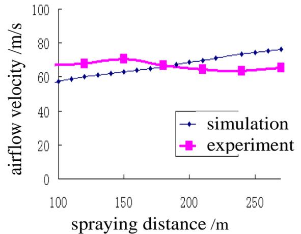
Fig. (16). The airflow velocity compares simulation with experimental value.
