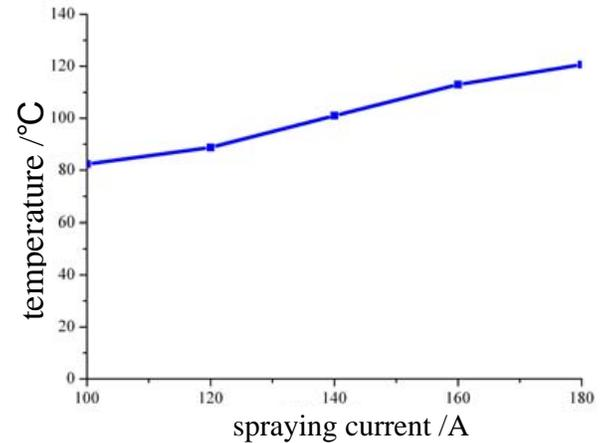
**Fig. (5).** The effect of spraying current on coating temperature.
