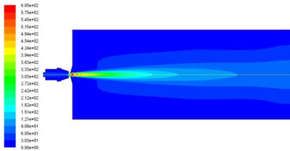
Fig. (6). Velocity field nephogram of melted metal airflow.
