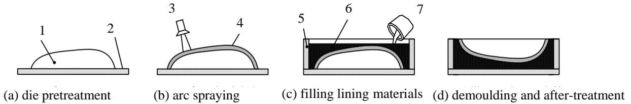
1- female die; 2- motherboard; 3- spraying gun; 4- metal coating; 5- frame; 6- lining material; 7- filling vessel
