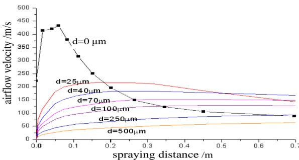
Fig. (11). The effect of different metal grain diameter on airflow velocity.
