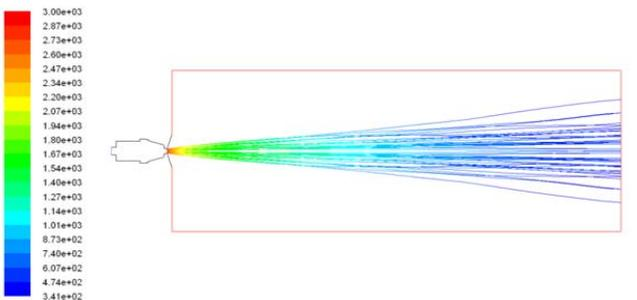
Fig. (9). Temperature distribution nephogram of melted metal airflow.
