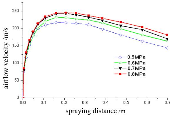
Fig. (10). The effect of different air pressures on airflow velocity.
