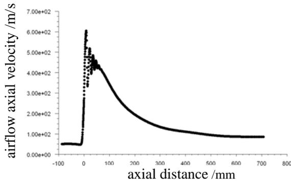
Fig. (7). The change of airflow axial velocity along with axial distance.
