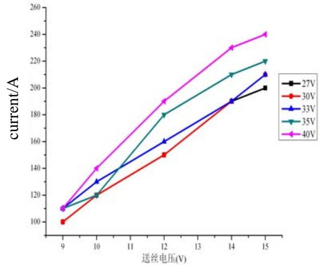
**Fig. (4).** The influence of wire feed voltage on arc current.
