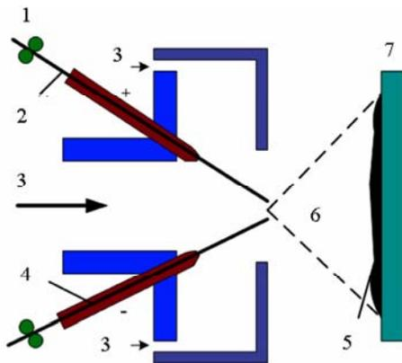
**Fig. (1).** The arc spraying principle. 1- wire feeder; 2- electric conduction wire; 3- compressed air; 4- nozzle; 5- spraying coating; 6- melted metal drop; 7- die surface.
