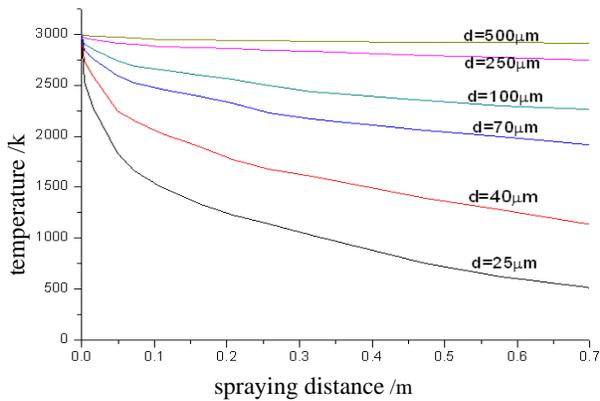
Fig. (13). The temperature distribution of grains under different diameter along with jet flow axis.
