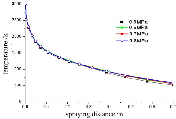
Fig. (12). The temperature distribution of grains under different pressures along with jet flow axis.
