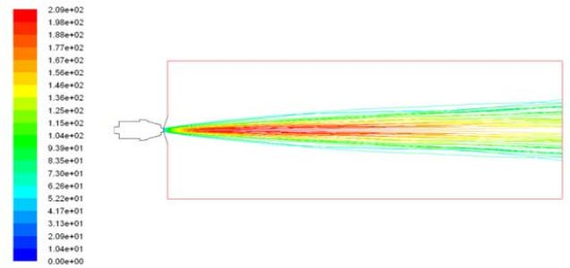
Fig. (8). Velocity distribution nephogram of melted metal airflow.
