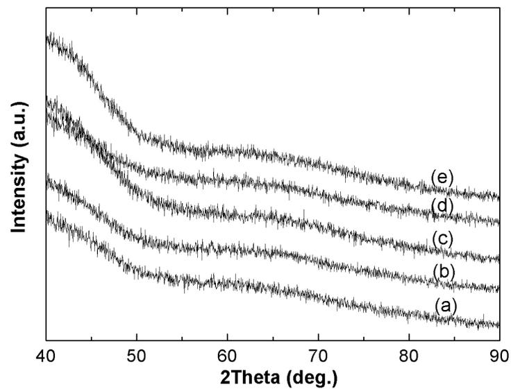
Fig. (3). X-ray diffraction patterns of the  $Co_{1-x}P_x$  alloy nanowires with  $x=6.8$  wt% for different diameter: (a) 10 nm; (b) 40 nm; (c) 80 nm; (d) 100 nm; (e) 130 nm.
