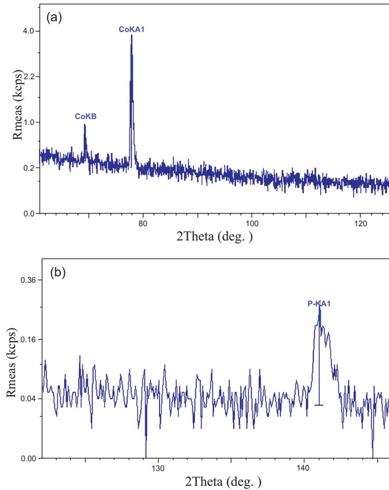
Fig. (2). XRF analysis of the  $Co_{1-x}P_x$  alloy nanowires with  $x=6.8$  wt%.
