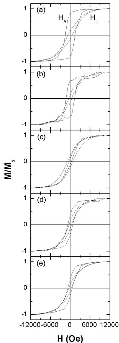
**Fig. (5).** Hysteresis loops of the  $\text{Co}_{1-x}\text{P}_x$  alloy nanowires with  $x=7.6$  wt% for different diameter at ambient temperature: (a) 10 nm; (b) 40 nm; (c) 80 nm; (d) 100 nm; (e) 130 nm.  $H_{//}$  and  $H_{\perp}$  represent that the applied field  $H$  are parallel and perpendicular to the wires axis.
