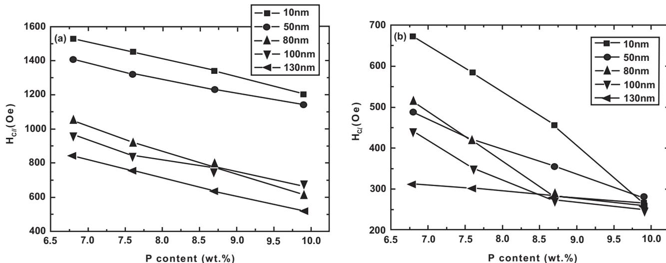
**Fig. (6).** The dependence of the nanowire arrays coercivity on P content for different diameter: (a)  $H_{c//}$ ; (b)  $H_{c\perp}$ .  $H_{c//}$  and  $H_{c\perp}$  represent the coercivity of the applied field  $H$  are parallel and perpendicular to the wires axis.
