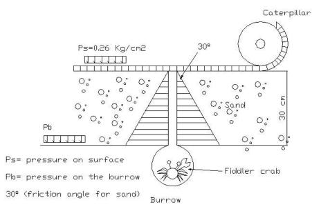
Fig. (6). The pressure over the burrow walls diminishes according to the internal friction angle of the sand. The fiddler crab only support the tidal water level pressure.
