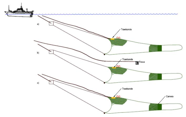
Fig. (1). The methodology employed in the three surveys included,  $\mathbf{a}$ ) a trawl-sonde with echogram printouts (Method A),  $\mathbf{b}$ ) a trawl-sonde and a towed platform equipped with a sonar and a camera (Method B),  $\mathbf{c}$ ) a trawl-sonde with echogram printouts in combination with a video-camera inside the trawl belly (Method C).
