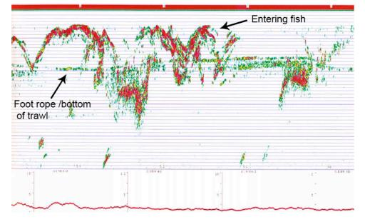
Fig. (2). Echogram from the trawl sonde taken from tow PT1261 in 1997, method A. The echogram shows fish entering the trawl. The continuous line just above the middle of the picture represents echoes from the foot-rope/bottom of the trawl. Some fish are passing under the foot-rope.
