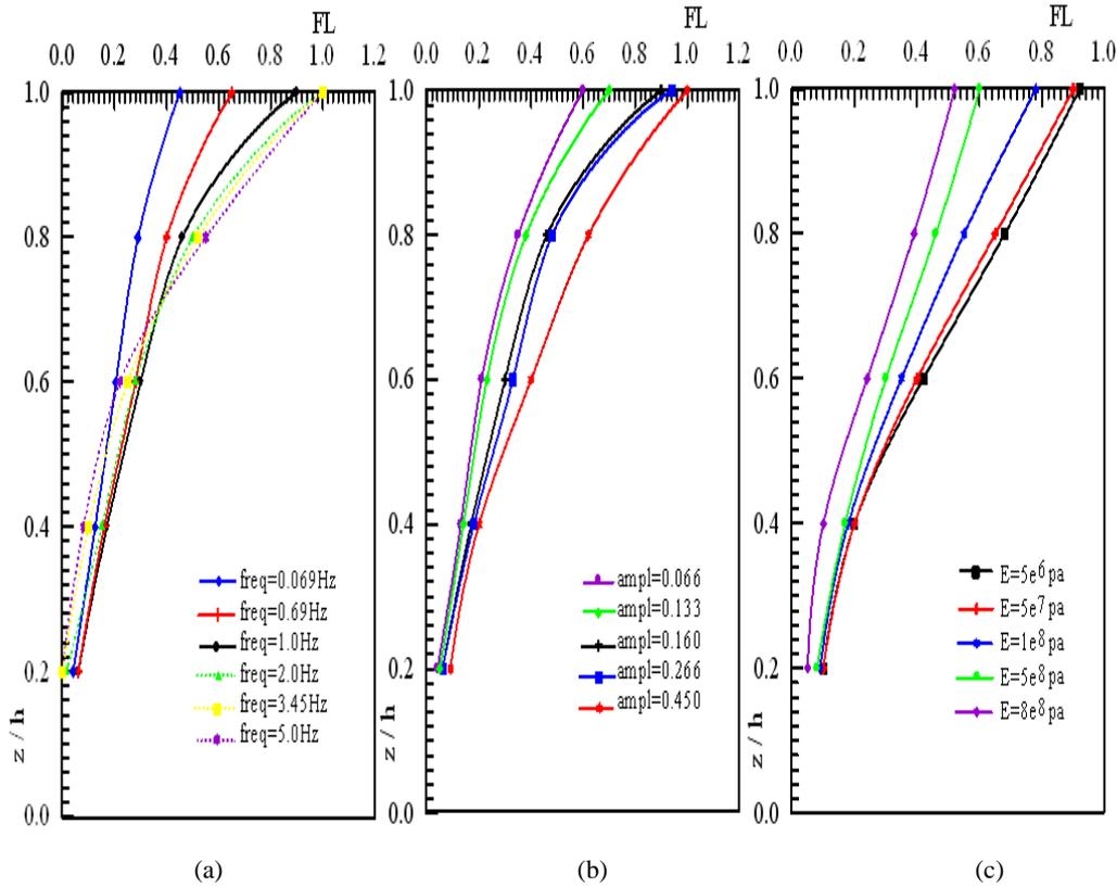
Fig. (8). Distribution of liquefaction degree and influencing factors.
