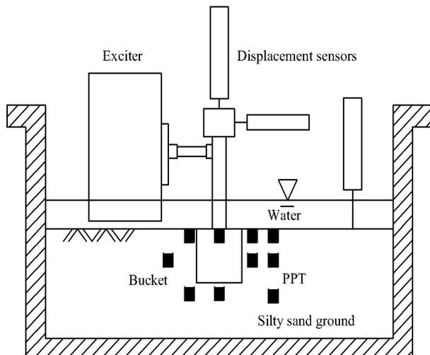
Fig. (1). Layout of centrifugal model.
