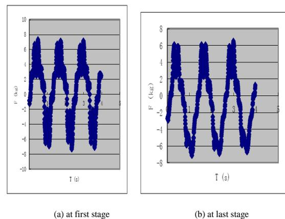
Fig. (3). Dynamic ice-induced load acts on the bucket.
