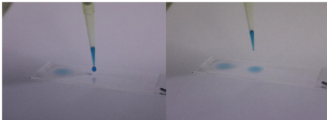
Fig. (5). Representative picture of spotting a product stained with dye methylene blue (0.1%) on a HCT-monolayer. Left picture: blue spot: first drop applied and second drop immediately before application. Right picture: the second drop spread immediately over the HCE-T monolayer surface.
