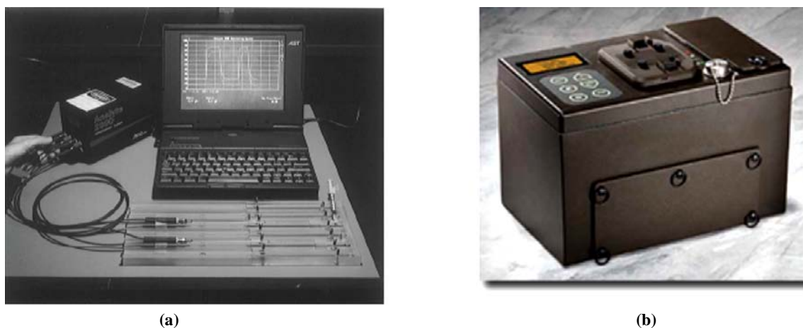
Fig. (2). Fiber-optic biosensors developed by Naval Research Lab in collaboration with Research International Inc. (a) Analyte 2000 portable fiber-optic biosensor. (b) User-friendly Raptor model for battlefield environment.
