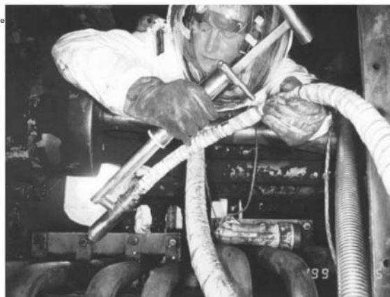
Fig. (5). A LIBS system with a 75 m all-fiber probe developed by Applied Photonics Ltd. (a) Principle of operation; (b) Deployment of the all-fiber LIBS probe inside a superheater.
