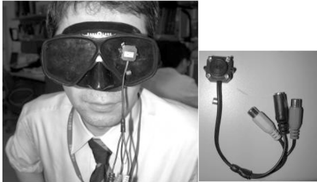
Fig. (2). Photograph of the CMOS camera with the handmade goggles. CMOS camera is securely equipped on the scuba diving goggles.
