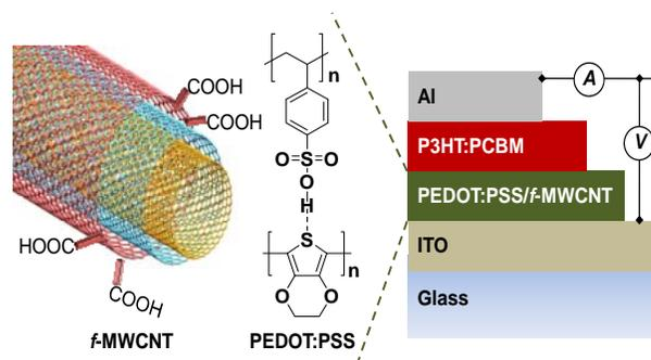
**Fig. (1).** Illustration of device structure and chemical structures of *f*-MWCNT and PEDOT:PSS used for hole-collecting buffer layer.
