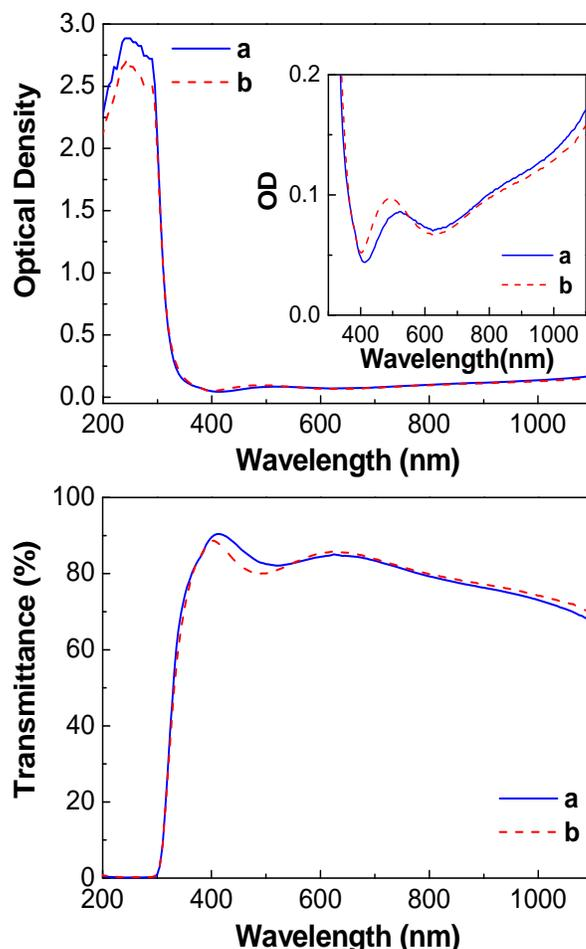
Fig. (2). Optical absorption (top) and transmittance (bottom) spectra of buffer layers coated on ITO-glass substrates: (a) PEDOT:PSS and (b) PEDOT:PSS/*f*-MWCNT. The inset (top panel) shows the enlarged spectra to find out the OD difference of the two samples.
