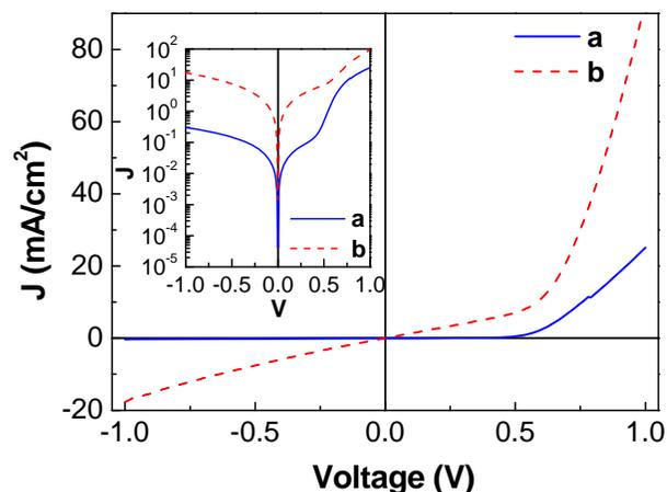
Fig. (3). Dark J-V characteristics of devices: (a) PEDOT:PSS and (b) PEDOT:PSS/*f*-MWCNT. Inset shows corresponding J-V curves on a semi-logarithmic scale.
