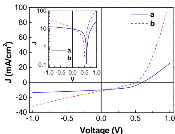
**Fig. (4).** Light (AM 1.5G, 100 mW/cm<sup>2</sup>) J-V characteristics of devices: (a) PEDOT:PSS and (b) PEDOT:PSS/f-MWCNT. Inset shows corresponding J-V curves on a semi-logarithmic scale.
