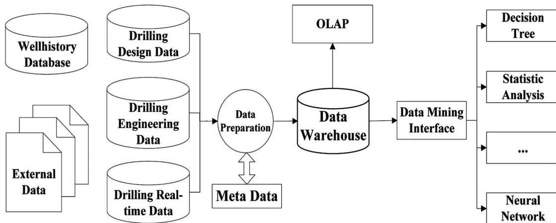
Fig. (1). System Architecture of Drilling Engineering Data Warehouse Solution.
