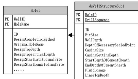
Fig. (3). Relation Diagram of Well Structure Design S1
