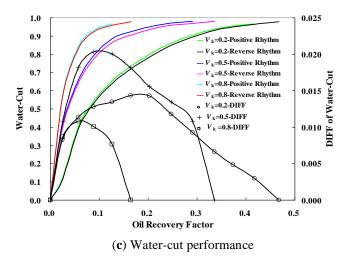
Fig. (13). Comparison of development characteristics for different sedimentary rhythm reservoirs.
