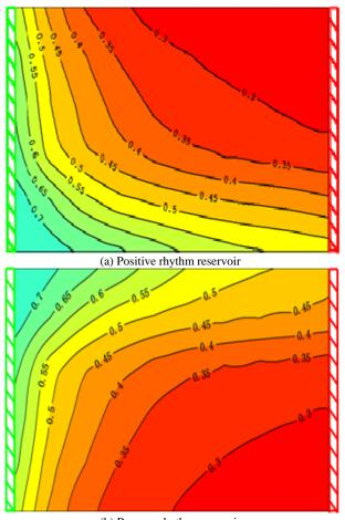
(b) Reverse rhythm reservoir **Fig. (7).** Formation water saturation profile when R=10% for  $V_{k}=0.53$ .
