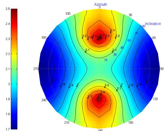
Fig. (7). Critical fracture pressure vs. well azimuth with original pore pressure.
