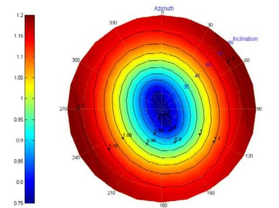
Fig. (8). Critical collapse pressure vs. well azimuth with depleted pore pressure (our model with horizontal stress reorientation).
