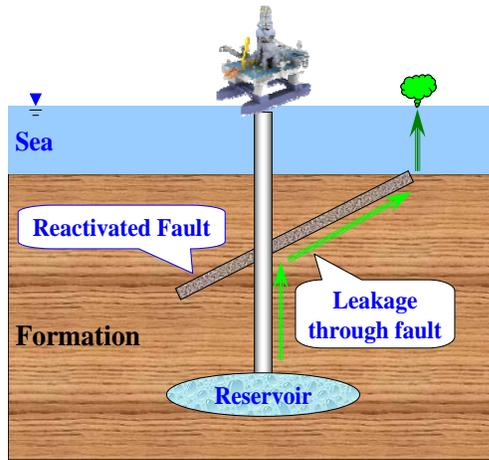
Fig. (1). Fault reactivation when drilling near the fault (Oilfield in Bohai Bay Basin).
