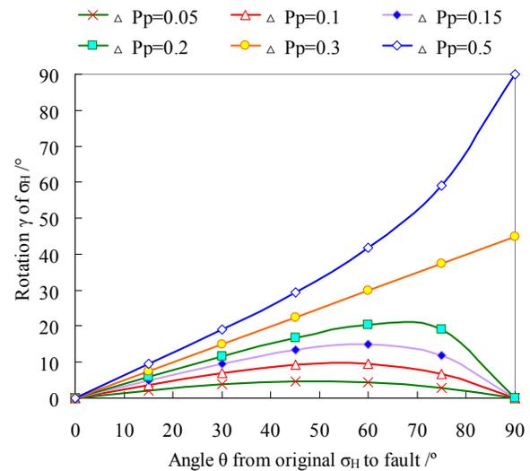
Fig. (3). Rotation angle ( $\gamma$ ) of horizontal stress orientation vs. the included angle ( $\theta$ ) between fault strike and original orientation of  $\sigma_H$ .
