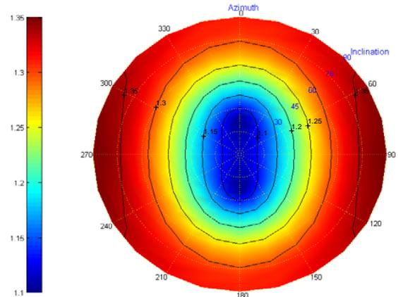
Fig. (6). Critical collapse pressure vs. well azimuth with original pore pressure.
