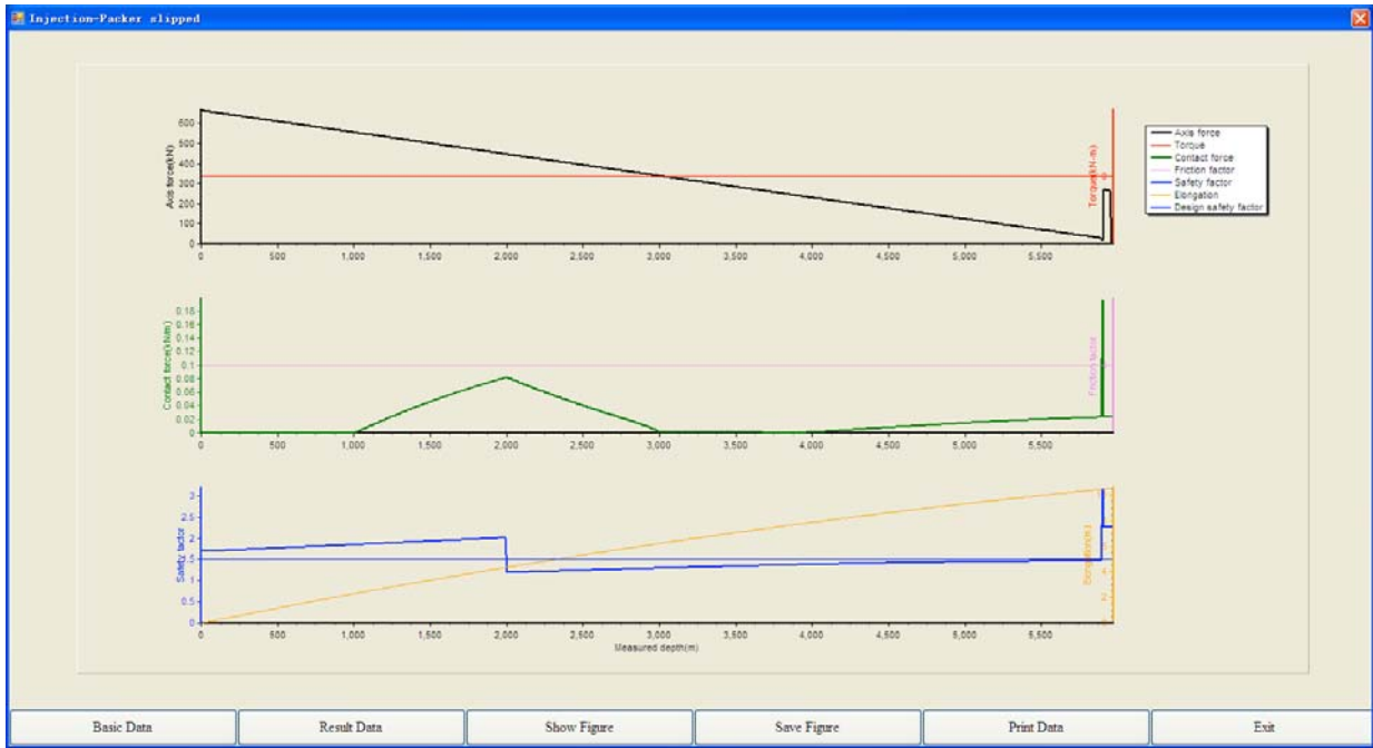
Fig. (4). Mechanical conditions of T-1 well string in injection.
