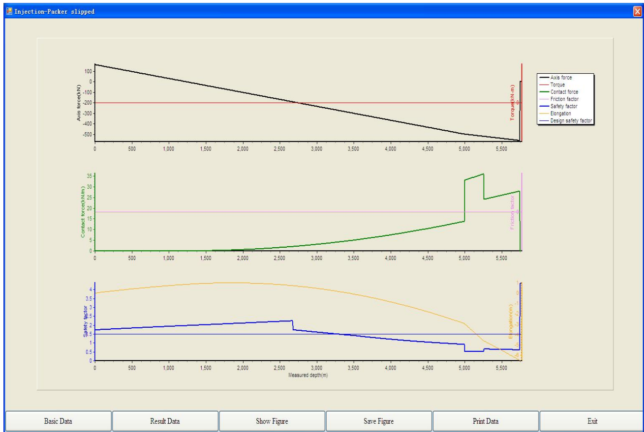
Fig. (2). Shows the mechanical conditions of S-1 well string while packer slipping upwards.
