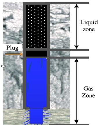
**Fig. (1).** The schematic of ideal wellbore model during bullheading process.
