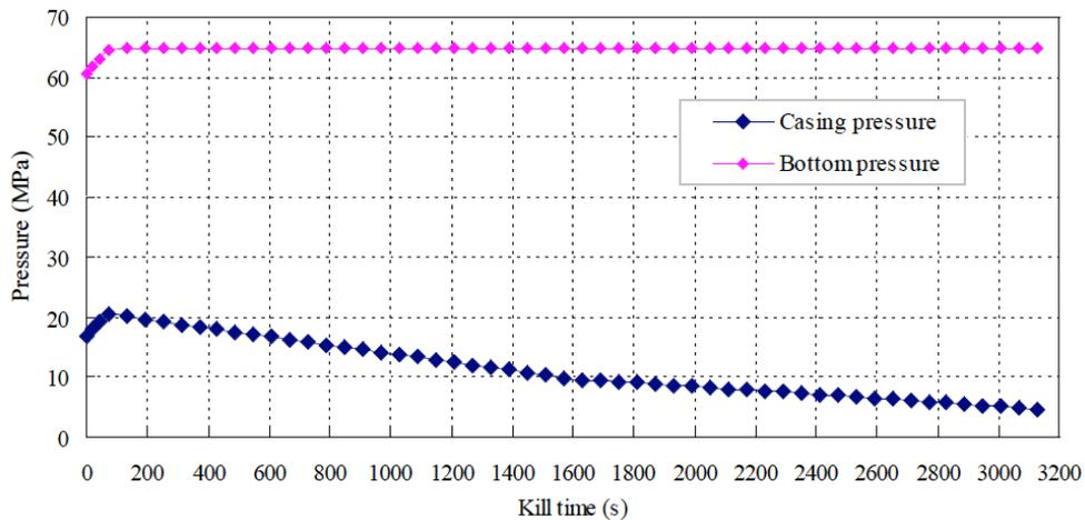
Fig. (4). The calculated results in terms of observed well casing and bottom pressure.
