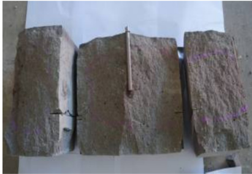
Fig. (9). The fracturing results of laboratory test of group 2 cores.
