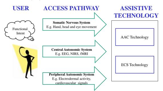
Fig. (1). Potential access pathways for the translation of functional intent into the control of assistive technologies (AAC = augmentative and alternative communication; ECS = environmental control system).
