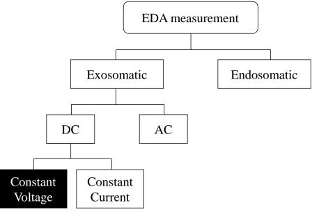
Fig. (3). The categories of potential EDA recording techniques. The most popular measurement technique in the literature is highlighted.
