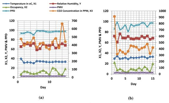
Fig. (4). Indoor RH, temperature, occupancy and  $CO_2$  concentration for Husky Foods in the (a) morning; and (b) afternoon (The horizontal axis depicts the days, while the primary vertical axis depicts the temperature in degrees Celsius, relative humidity in %, occupancy, PMV and PPD; while the secondary vertical axis shows the  $CO_2$  concentration in PPM).
