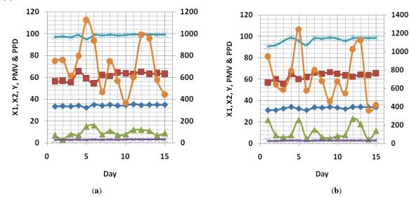
Fig. (9). Indoor RH, temperature, occupancy and  $CO_2$  concentration for Pinto Lounge in the (a) morning; and (b) afternoon. Other details are as in Fig. (4).
