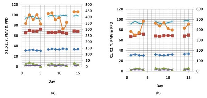
Fig. (6). Indoor RH, temperature, occupancy and  $CO_2$  concentration for Hommies Bakery in the (a) morning; and (b) afternoon. Other details are as in Fig. (4).
