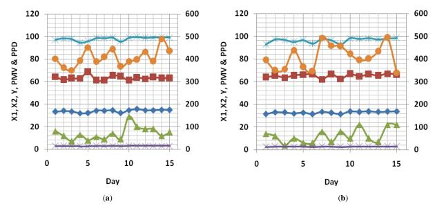
Fig. (8). Indoor RH, temperature, occupancy and  $CO_2$  concentration for Wisdom Cafe in the (a) morning; and (b) afternoon. Other details are as in Fig. (4).
