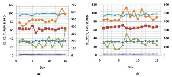
Fig. (7). Indoor RH, temperature, occupancy and  $CO_2$  concentration for Eatery Hall in the (a) morning; and (b) afternoon. Other details are as in Fig. (4).
