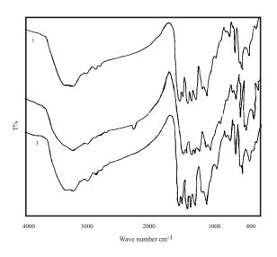
**Fig. (6).** Infrared spectra of untreated and treated Nomex fabric with CD-T or CD-T.
