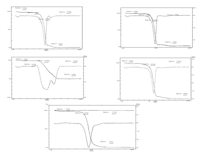
Fig. (3). Thermogravimetric analysis (TGA) of polyamide 6 fabric. a) Untreated b) Treated with CD 30g/l c) Treated with CD 50g/l d) Treated with CD-T 30g/l e) Treated with CD-T 50g/l.
