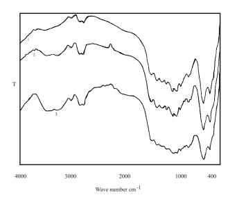
**Fig. (4).** Infrared spectra of untreated and treated polyamide 6 fabric with CD-T or with CD-T.
