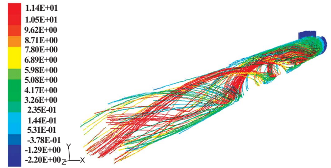
Fig. (7). The axial velocity path lines for a single microtube mass flow rate M = 110 \cdot 10^{-5} kg/s.
