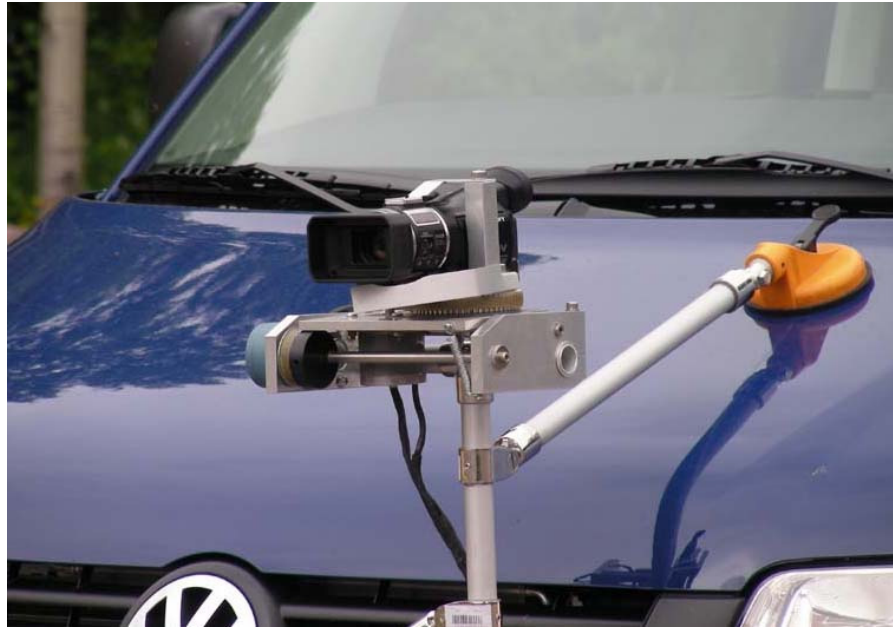
Fig. (2). Video camera mounted in front of the vehicle. The camera is operated from the cabin; the recording describes how visibility towards the railway improves as the vehicle approaches the level crossing.
