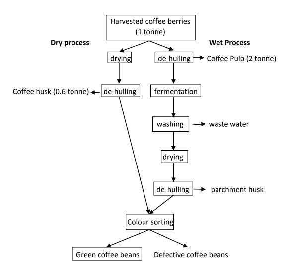
Fig. (2). Coffee processing and residues produced (adapted from Ghosh and Venkatachalapathy [6]).
