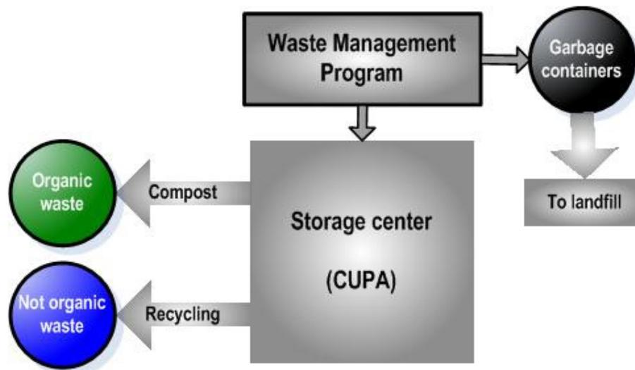
**Fig. (1).** Operation diagram of the storage center and destination of the waste.
